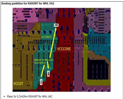
Figure 11-11. Whiskey Lake U 4+2/Coffee Lake U 4+2f/Cannon Lake U 2+2/ Coffee Lake U 4+3e Processor - RSHUNT Routing and Placement Guideline
